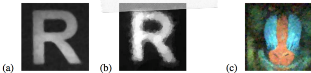
Fig. 2. Single-pixel photo album. (a) 256 \times 256 conventional image of a black-and-white R. (b) Single-pixel camera reconstructed image from M = 1300 random measurements ( 50\times sub-Nyquist). (c) 256 \times 256 pixel color reconstruction of a printout of the Mandrill test image imaged in a low-light setting using a single photomultiplier tube sensor, RGB color filters, and M = 6500 random measurements.
