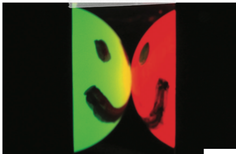
Fig. 4. (Color online) Scene consisting of a Ping-Pong ball illuminated by a 543 nm green laser and a white light source through a 560 nm narrowband filter (left), and a red Ping-Pong ball illuminated by a white light source (right).
